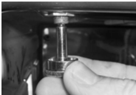
Keep the metal cover in a safe place when using the meat probe, as this will need to be re-inserted for use in other cooking modes.
