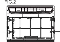
3. Locate the four Front Panel screws and remove. These screws will be needed to re-install the Front Panel later (See FIG.2).
