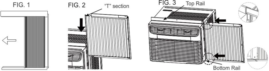
Your air conditioner is designed to install in standard double hung windows with opening widths of 24 to 36 inches (610 mm to 914 mm) (FIG. 4A, FIG. 4B). Lower sash must open sufficiently to allow a clear vertical opening of 14 inches (356 mm).
