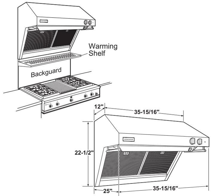
Each hood is shipped with a stainless steel backguard and a warming shelf. Hoods may be installed with the shelf or backguard alone, or with both as shown.
