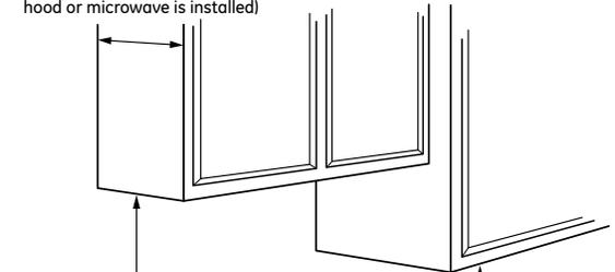
30" MIN. from countertop to unprotected cabinet (when no hood or microwave is installed)
