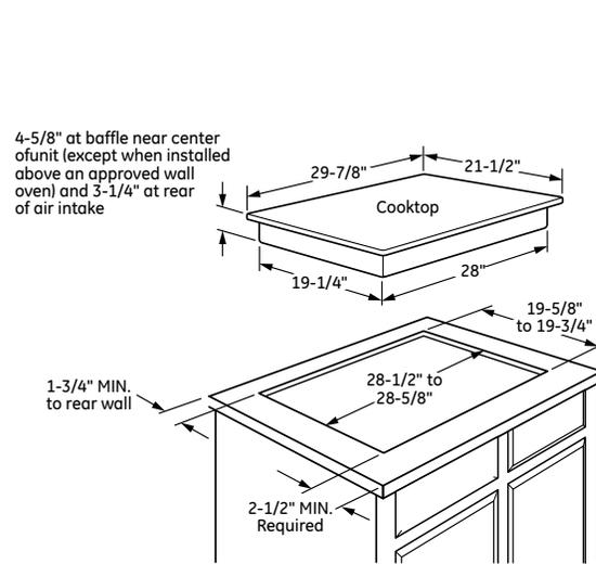
To insure accuracy, it is best to make a template when cutting the opening in the counter
