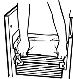
2. Lock bag in place by pulling the 4 prepunched holes over the bag retainer buttons. Holes will expand over the buttons without damaging the bag.
