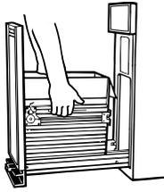
4. Vacuum the inside of the cabinet. Liquid spills or wet trash should be cleaned up by hand, or by using a vacuum cleaner designed to pick up liquids.
