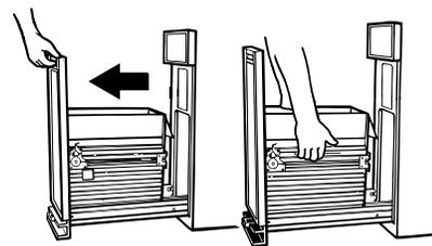
11. Place the other 2 corner posts on the floor to the side of the compactor.
