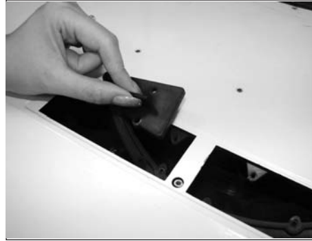
6. Remove (2) interior recirculating panels.
