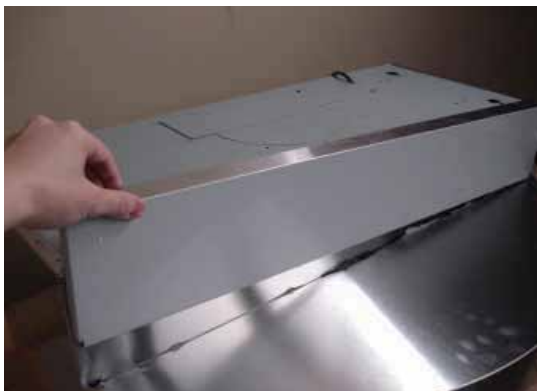
For Tamburo (ZTA) and Terazzo (ZTE) only: Unscrew and remove the front cover
